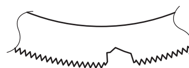
Damage of Saw Blade
