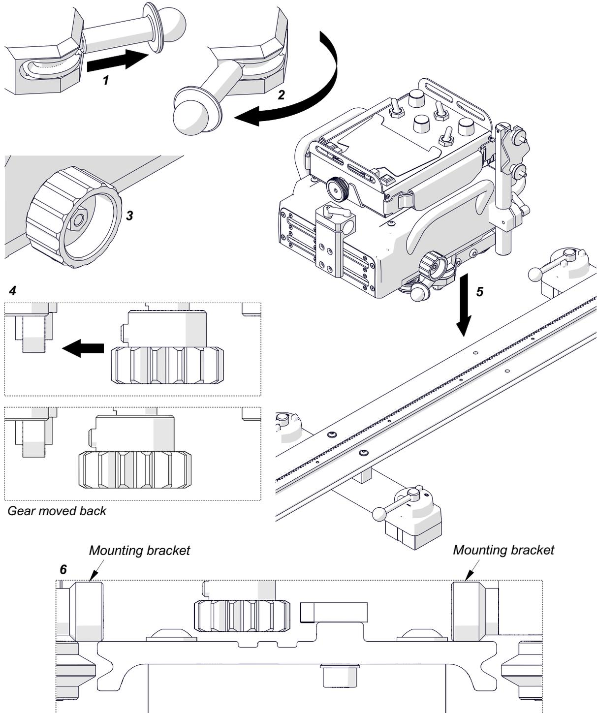
Set the lever to ON (1) to put the rollers into the grooves (2). Tighten the knob (3) to engage the gear of the carriage with the rack of the rail (4). Keep a small backlash between the gear and the rack. Move the carriage slightly back and forth to make sure that there is a backlash.
