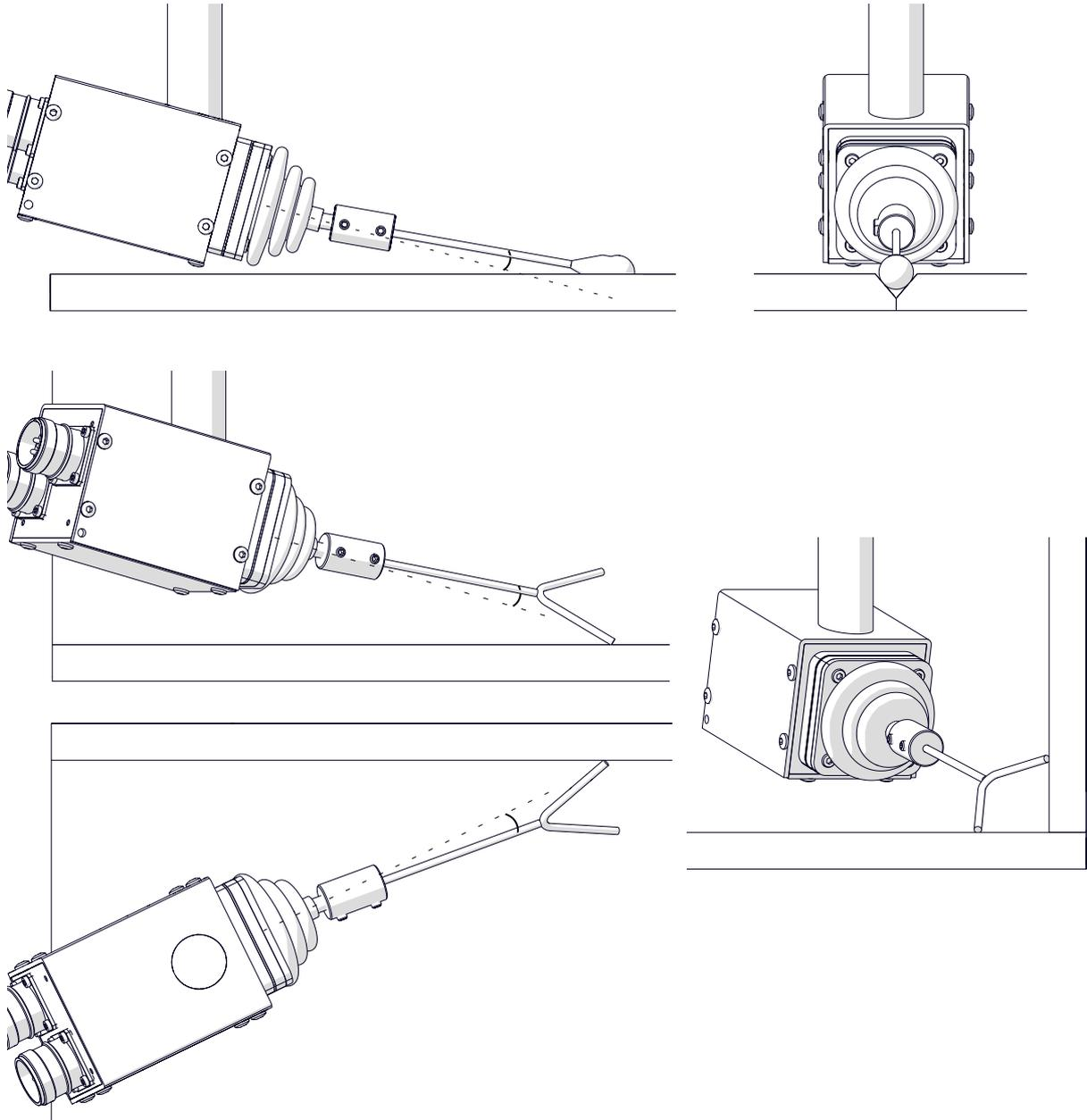
The figure shows how the tracking system works. When the tip of the sensor moves, the system senses any small change in position of the seam. Then, the oscillator, the vertical slide, and the torch, are moved to maintain the correct position above the seam.
