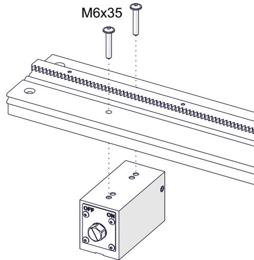
To clamp the unit to the surface, use the 17 mm flat wrench (not included) and set the side screw to ON.
