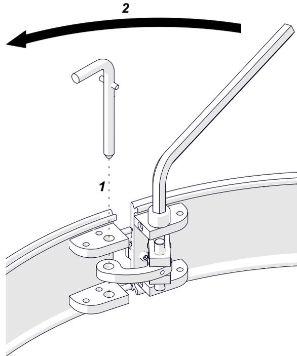
Use the 13 mm flat wrench to adjust the bolts (or the screws by hand) until they are in contact with the workpiece (1). Adjust each support equally to make the track concentric to the workpiece. Lock the supports with the nuts (2) or levers.
