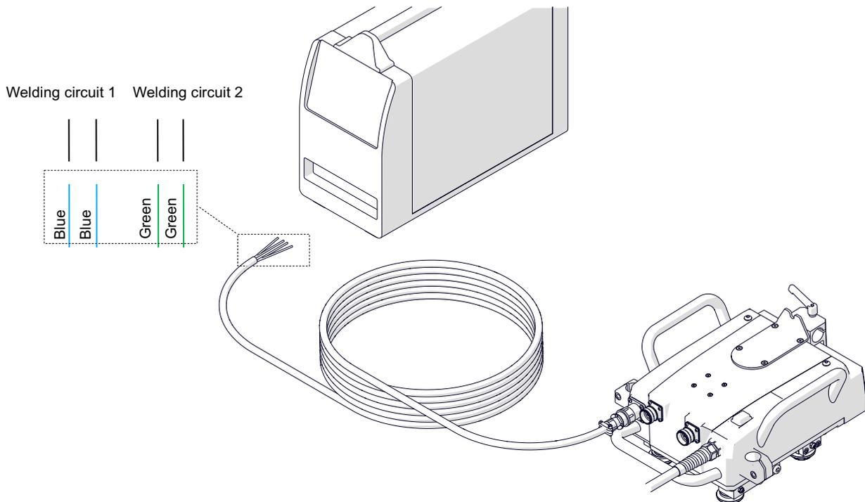
Make sure that the arc ignition cable is connected correctly. To do this, turn on the power of the carriage, and then set the arc ignition switch to TEST. This should enable the arc for a while.
