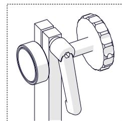
Put the workpiece vertically, and then put the rails onto the workpiece so that the teeth of the racks point down. Next, for all rails, use the 12 mm hex wrench to set the hinge as shown. Then, put the lock pin through the holes (1), and then rotate the wrench (2) to connect the rails.
