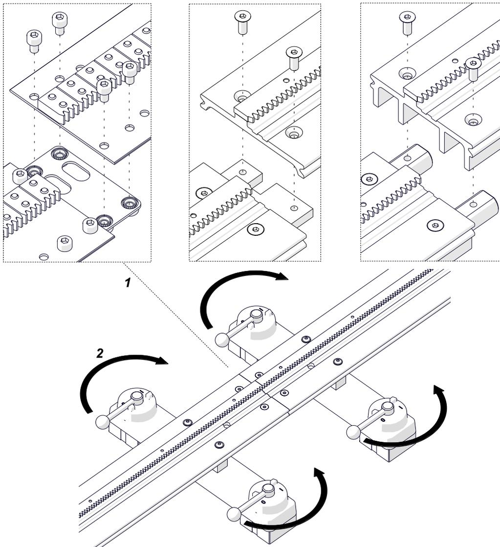
If a semi-flex rail is put on a curve, before you attach more rails use the 4 mm hex wrench to loosen the screws of the connecting plates (1) and of the racks (2). Next, attach the rails, clamp them with levers, and then tighten the connecting plates. Put the rack adjustment tool (not included) into the hole (3), and rotate the tool to the left (4) to remove the gap (5) between the racks. Then, tighten the leftmost screw and the rightmost screw of each rack (2).
