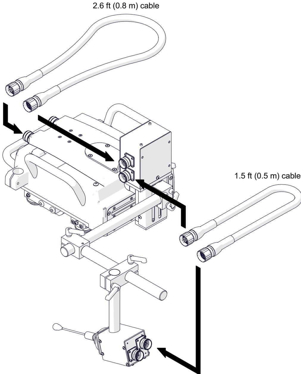
Install the torch into the torch holder. Then, tilt the rod of the sensor against the workpiece so that there is tension in the rod. Next, put the tip as shown.
