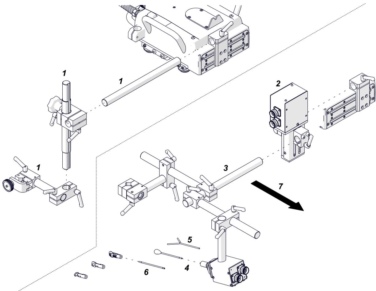
Use the 2.6 ft (0.8 m) cable to connect the motorized vertical slide to the carriage. Then, use the 1.5 ft (0.5 m) cable to connect the sensor to the vertical slide. If the vertical slide is not used, connect the sensor to the carriage with the 3 ft (1 m) cable.
